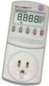
To assess an appliance’s energy use, just plug the Kill A Watt into a wall outlet and then plug an appliance into the monitor. A large LCD display counts consumption by the kilowatt-hour, and you can figure out your electrical expenses by the hour, day, week, month or even an entire year. You also can monitor the quality of your power by displaying voltage, line frequency and power factor.
